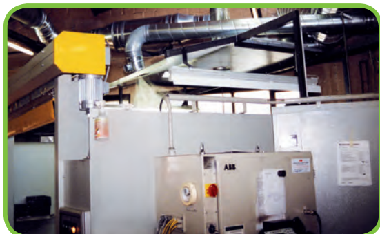
◀ Robot extraction hoods in various versions, e.g. with edge extraction or only as nozzle panel, customized.
