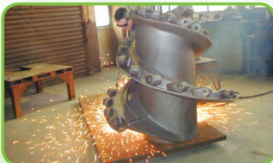
◀ Extraction table with water bath for flame cutting, available in various sizes.
