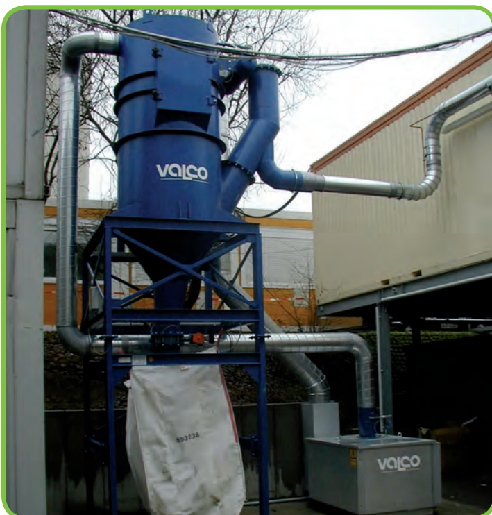
▼ Central high vacuum extraction and filter system, explosion-proof, 3500 m 3 /h, 25 kPa, 45kW, for the extraction of epoxy resins and cotton fluff, chemical industry.
