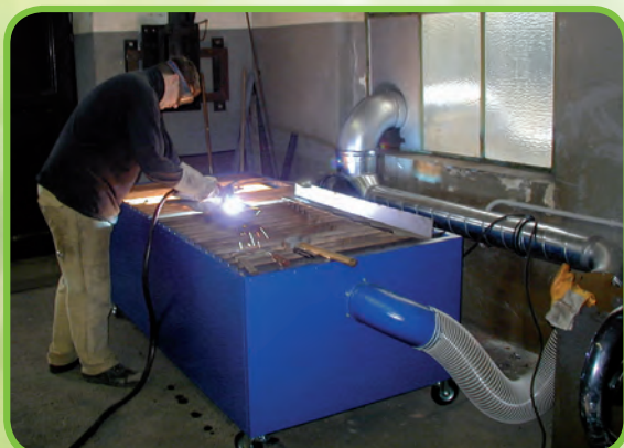
◀ Extraction table with water bath for flame cutting, available in various sizes.
