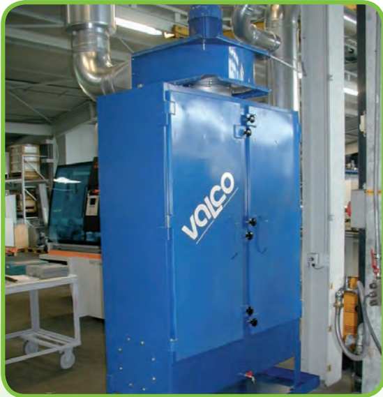
▼ Dust extraction system with bag filters for 40,000 m 3 /h, cast steel foundry
