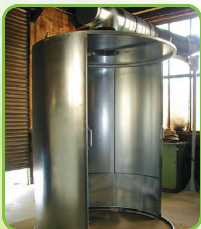
◀ Rotatable extraction hood for flame cutting, customized ▼
