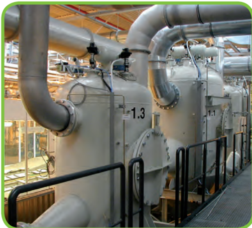
ATEX-cartridge filter, 11 bar pressure-resistant for explosive powder
